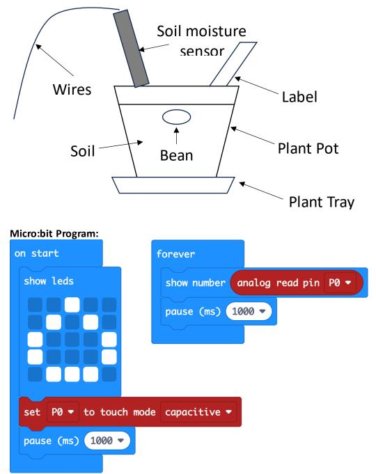
Note, if using the sensor from the starter kit, remove the block to set P0 to touch mode capacitive.
